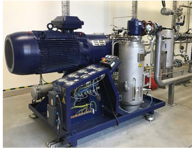
Photo 4. Biogas Purification System absorbing carbon dioxide
